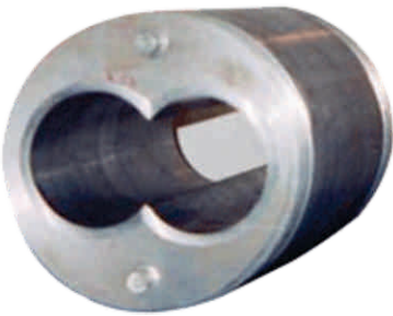
VARIOUS TYPE OF SLEEVES FITTED FRONT BARREL
